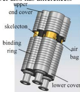
Fig.1 Pneumatic flexible joint structure
